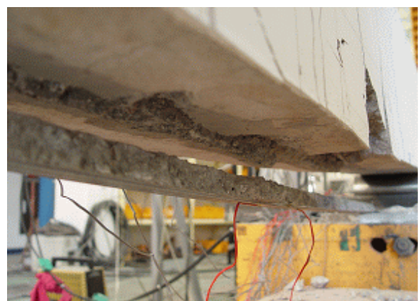
Fig. 6 Near surface mounted method using
