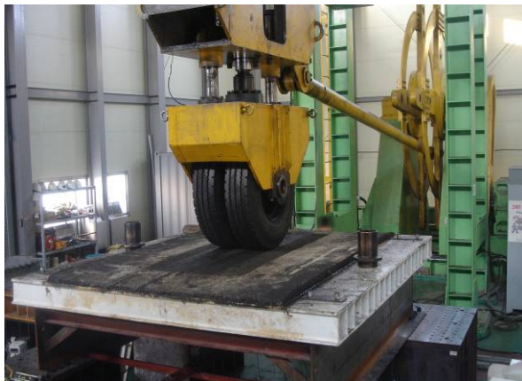
Fig. 21 Wheel rolling test of bridge pavement for FRP deck
