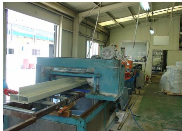
Fig. 4 Pultrusion of deck panel
