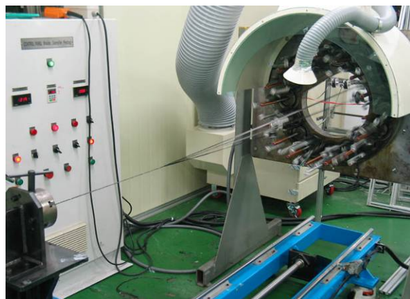
Fig. 11 Braiding of FRP rebar
