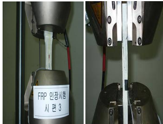
Fig. 20 Fatigue test of FRP material
