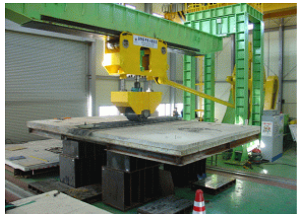
Fig. 25 Moving wheel load test of FRP-Concrete composite deck
