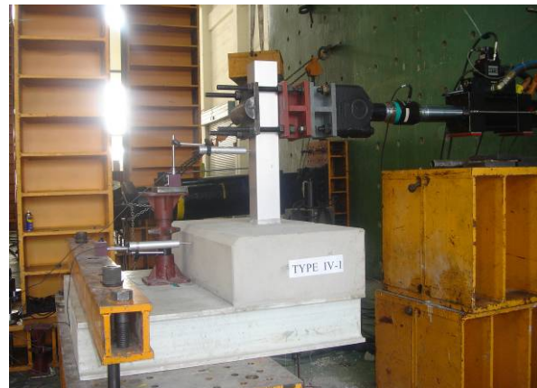
Fig. 22 Performance test of parapet
