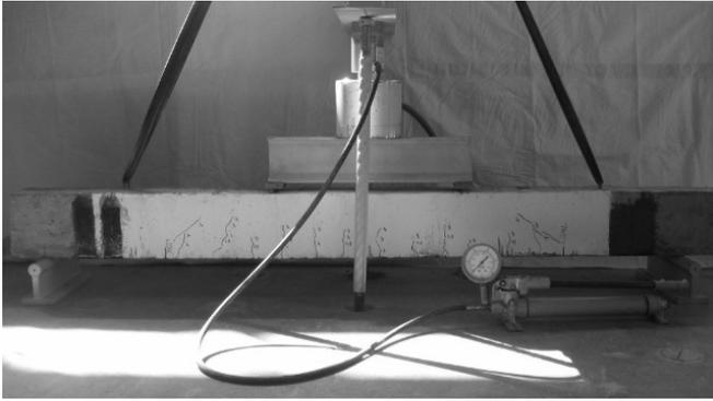
Figure 2. Static loading setup.
