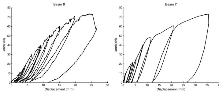
Figure 3. Load-displacement diagram for beams B6-16D-2L and B7-12D-1L.
