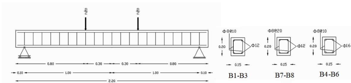
Figure 1. Specimens (Dimensions are in meter).
