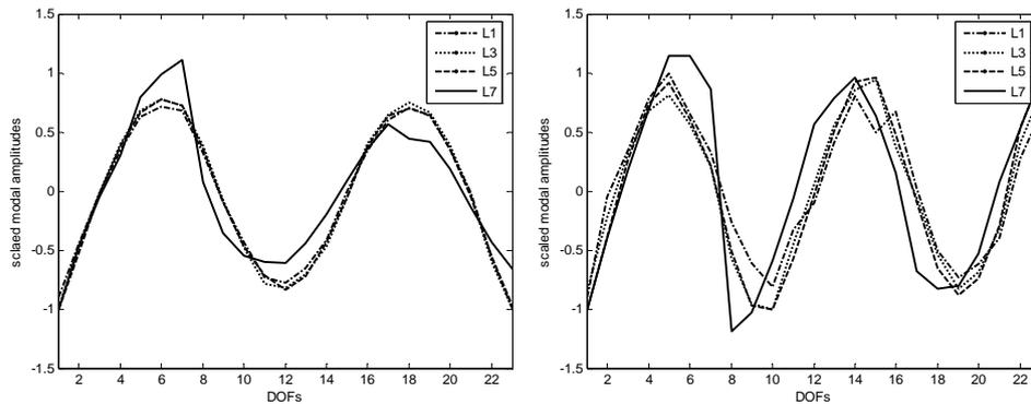
Figure 9. The third and the fourth mode shapes of beam B5-16D-2L-W in various steps.
